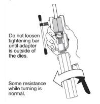
8) Loosen the tightening bar and remove the tube. It should look something like the sketch below.
