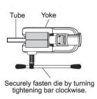
Grasp the yoke and rotate the hydraulic cylinder clockwise until it stops.
