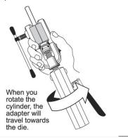
5) Begin squeezing the lever and continue until the edge of the adapter meets the die or pumping action shows substantial resistance.
